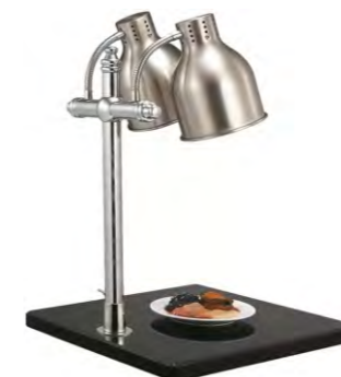
MWLM02H 220-240V, 50/60Hz, 250Wx2, 550 x 500 x (h)750mm
